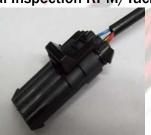
On the same harness leg as the Chassis Harness Connector or Switch Wires, another optional item is the standardized U6SA RPM Plug. This connection contains provisions for a tachometer to be connected using a professional connector. Without a tachometer, the plug contains a "dead end" cap to prevent dirt and moisture contamination.
