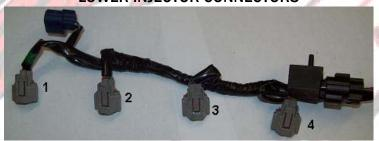
The lower injector sub-harness features not only the four injector connectors but also two air pressure sensors. The blue connector is for the Intake Air Pressure sensor and must be connected to a vacuum line from the throttle bodies.
