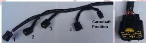
The large plug on the right is the main connector for the ignition coil sub-harness. It connects the ignition coils to the main engine harness. The photo on the left shows the individual ignition coil connectors at the other end of the sub-harness. These connectors are each 2pin connectors. The Camshaft Position Sensor is a 3pin connector which connects to a corresponding 3pin connector coming from the engine valve cover.
