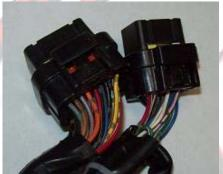
The ECU Connectors are some of the most identifiable because of the multitude of wires leading to them. These will be the largest and most populated connectors on the harness. On harnesses converted after Nov. 2010, two separate wires will be tied up near the ECU connector. These wires are for use with the Power Commander 5. Consult our Power Commander 5/Auto Tune Instruction Page for further information regarding the placement of these two wires.
